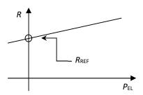
Now we have the information needed to find the temperature of the filament based on its resistance. Next, the same measurements we used for  $R_{\rm REF}$  can be used for determining  $K_{\rm LOSS}$ .
