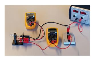
During the first measurements a resistor is placed in series connection with the lamp
