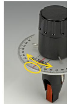
Vary the angle  $\theta$  in steps of  $10^\circ$  and note each time the reading of the scales. Write the angles with sign. If possible, measure from  $-100^\circ$  to  $+100^\circ$ .
