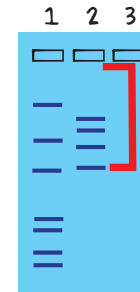
Figure 7: Measure distance migrated from the lower edge of the well to the lower edge of each band.
