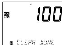
Logged data on edge® can be transferred from the meter to a USB flash drive by using the log recall function. The minimum requirement for the drive is USB 1.1. Select the pH, EC or DO record you wish to export and follow the simple steps below.
