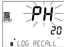
While the measurement type is blinking and message states "LOG RECALL", press CLR. "CLEAR ALL" and measurement type will be displayed with CFM tag blinking. Press CFM.
