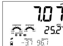
If measurements are taken successively in different samples, it is recommended to rinse the electrode thoroughly with deionized water or tap water and then with some of the next sample to prevent cross-contamination. The pH reading is affected by temperature. The temperature effect is compensated for using the temperature sensor inside the probe. The resulting measurement is the actual pH at the temperature of measurement.
