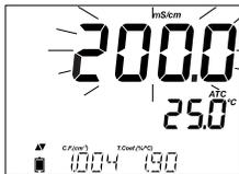
If the reading is out of range when the range is automatic, the full-scale value (200.0 mS/cm for ATC mode or 500.0 mS/cm for absolute conductivity) will be displayed blinking.
