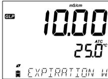
Calibration Expiration status together with the current reading:
