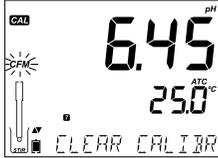
Press CAL then press CLR. "CLEAR CALIBRATION" will be displayed. Press CAL to exit calibration if you want to keep old calibration data instead of clearing.
