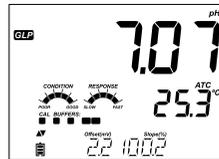
The last calibration date (yyyy.mm.dd) together with the current reading.
