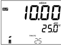
The reference temperature together with the current reading.
