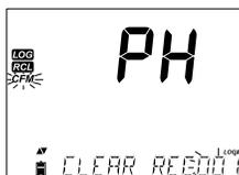
The instrument will display "CLEAR REC." and record number along with "CFM" tag blinking. Use the ARROW keys to select another record if necessary.
