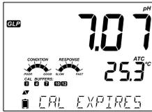
Or if enabled the number of days until the calibration alarm “CAL DUE” will be displayed. (i.e. CAL EXPIRES IN 2 DAYS)
