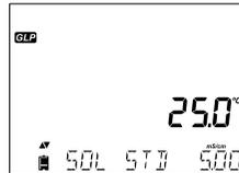
The temperature coefficient set at the calibration moment together with the current reading.
