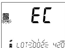
The display will return to the selected file. Press the RCL key twice to return to measurements.
