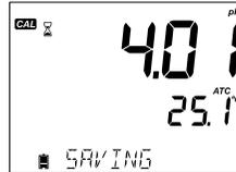
Each time a buffer is confirmed, the new calibration data replaces the old data for the corresponding buffer or for any near buffer in a ±0.2 pH proximity. If current buffer has no previous data stored and the calibration is not full (five buffers), the current buffer is added to the existing calibration. If the existing calibration is full, the instrument asks which buffer to replace.
