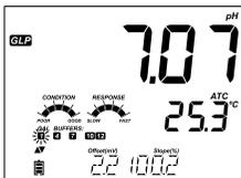
If a buffer is not from the last calibration, the buffer tag will be displayed blinking.
