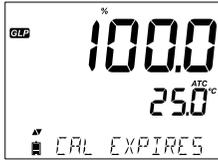
If enabled, the number of days until the calibration alarm "CAL DUE" will be displayed. (i.e. CAL EXPIRES IN 2 DAYS)
