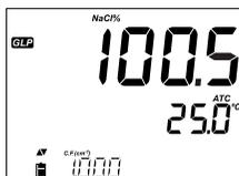
The salinity coefficient determined from the calibration together with the current reading.
