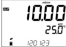
The last calibration time (hh:mm:ss) together with the current reading.
