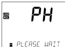
For Interval lots, the message "Clear", followed by the selected lot will be displayed with "CFM" tag blinking. Press the ARROW keys to select a different lot. Press CFM. The instrument will display "PLEASE WAIT".
