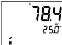
The Dissolved Oxygen value (in %) is displayed on the 1st LCD line and the temperature on the secondary LCD.
