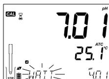
The calibrated value will be displayed on the 1st LCD line and the second expected buffer value on the 3rd LCD line.
