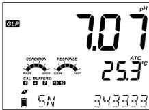
The probe serial number together with the current reading.
