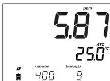
Press RANGE to change the reading from % to ppm (mg/L) and vice versa.
