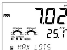
If the log memory is full during any logging session, the “LOG FULL” message will be displayed on the 3rd LCD line for a brief moment and logging will cease. The display will return to the measurement screen.
