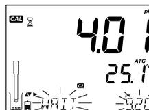
**Note:** Custom buffer value can be adjusted in a  $\pm 1.00$  pH window around the set value during calibration. When a custom buffer is displayed, the "C1" or "C2" tag is displayed.
