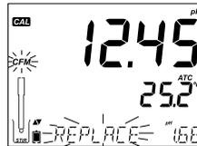
Press the ARROW keys to select another buffer to be replaced. Press CFM to confirm the buffer that will be replaced. Press CAL to leave calibration without replacing.
