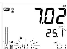
The "CAL" tag will appear and the "7.01" buffer will be displayed on the 3rd LCD line. If necessary, press the ARROW keys to select a different buffer value. The "WAIT" tag along with "STIR" tag will be displayed and "WAIT" will blink on the LCD until the reading is stable.
