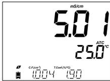
The conductivity value will be displayed on the 1st LCD line, the temperature on the 2nd LCD line and calibration or range specific information on the 3rd LCD line.
