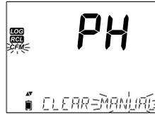
The lot number is used to identify particular sets of data. The lot numbers are allocated successively until 100, even if some lots were deleted. The total number of lots that can be saved is 100. If some are deleted (for example 1-50), fifty additional logs may be stored. These will be numbered 101-150. The lots are allocated successively (provided available memory space) until 999 is reached. After this, it is necessary to delete all the LOT logs to start over the numbering.
