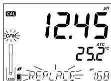
**Note:** Each time a buffer is confirmed, the new calibration data replaces the old data for the corresponding buffer or for any near buffer in a  $\pm 0.2$  pH proximity. If the current buffer has no previous data stored and the calibration has not used five buffers, the current buffer is added to the existing calibration. If the existing calibration is full, the instrument asks
