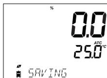
The instrument will display "SAVING" message and it will return to measurement mode. Rinse probe tip off in water before taking measurements in samples.
