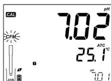
When the reading is stable and close to the selected buffer, "CFM" tag will blink. Press CFM to confirm calibration.
