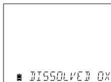
During this process, the following message will be displayed on the LCD, "DISSOLVED OXYGEN PROBE CONDITIONING".
