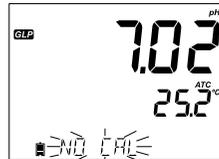
The pH calibration offset and slope (the GLP slope is the average of the calibration slopes; the percentage is referenced to the ideal slope value at 25° C). The condition and response show are from the last calibration.
