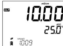
The calibration offset factor in  $\mu S/cm$  together with the current reading.
