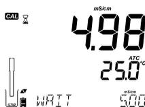
When the reading is stable and close to the selected standard, "CFM" tag will blink, the message "SOL STD" and the value will scroll.
