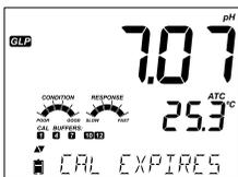
In Standard Mode, Condition and Response gauges are visible on the day of calibration (See Electrode Condition And Electrode Response Time page 24). If configured in SETUP, a countdown message displays the number of days remaining until a new Calibration is due.
