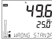
If the temperature goes out of (0.0 - 50.0 °C) range during calibration, the "WRONG STANDARD TEMPERATURE" message will be displayed and temperature value will blink.
