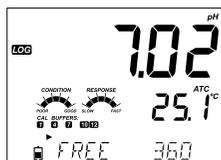
Pressing ► during an interval log will display the number of logs available.
