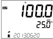
The date of the calibration together with the current reading.
