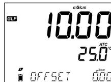
The Solution Standard and calibration temperature.
