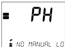
If no data was logged for the selected measurement range, the instrument displays the following messages (ex. for pH range):
