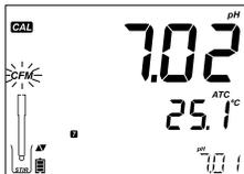
When the reading is stable and close to the selected buffer, the “CFM” tag will blink. Press CFM to confirm calibration.
